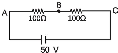
A voltmeter of resistance  $150 \Omega$  is connected across A and B. The potential drop across B and C measured by voltmeter is
